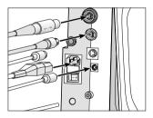
Connect the motor cable, operating controls, air hose, foot-operated starter (optional), coolant hose (control unit with external coolant supplying) and mains cable.
