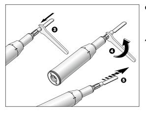
3 Guide the spanner to the clamping screw. Use the spanner to tighten the clamping screw.
