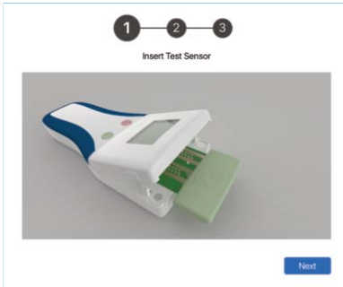
Figure 20: First step of the sensor test, insert the test sensor into the handheld
