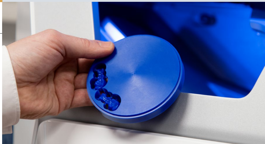
Milled result: Chip formation competitor product
