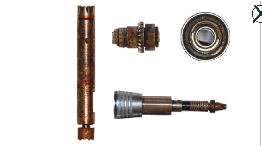
Improperly serviced handpieces
