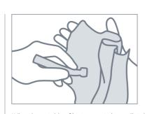
Wipe the outside of instruments immediately after the end of the treatment with an approved disinfectant. KaVo recommends the following disinfectants based on the compatibility of the materials:
