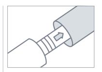
Remove the instrument from the motor coupling or the turbine from the MULTIflex quick coupler.
