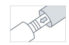
Prior to providing treatment, attach instruments and turbines onto the motor or MULTIflex coupling. Activate handpiece and let it run for a few seconds. Wipe off any escaping, residual lubrication oil. (Escaping, residual lubrication oil is common and does not damage dental instruments)
