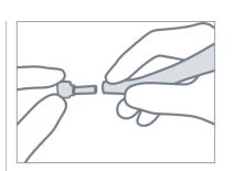
For instruments with interchangeable heads, remove the heads from the base for separate reprocessing.
